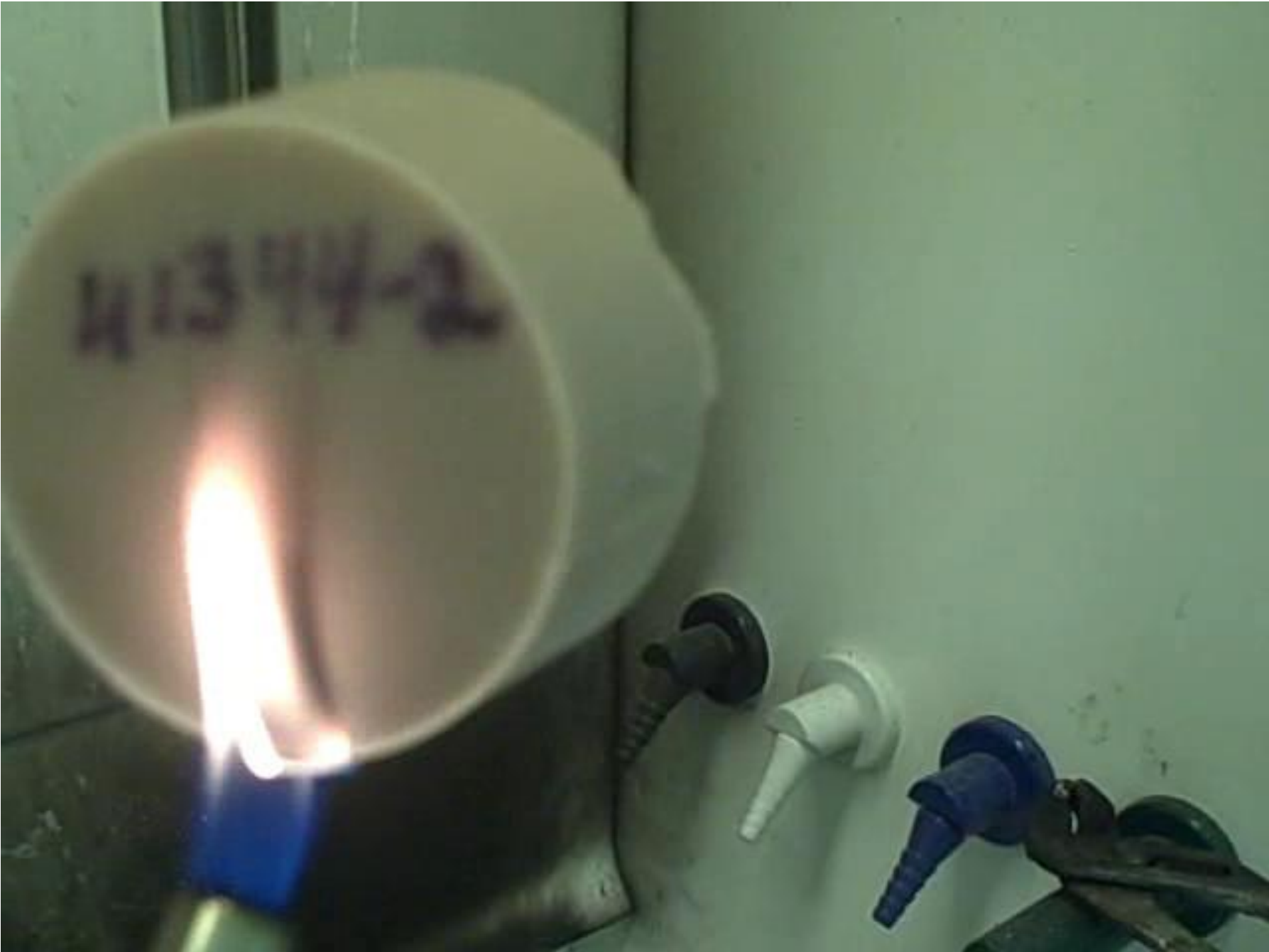
PVC emulsion FR treated to withstand open flames
